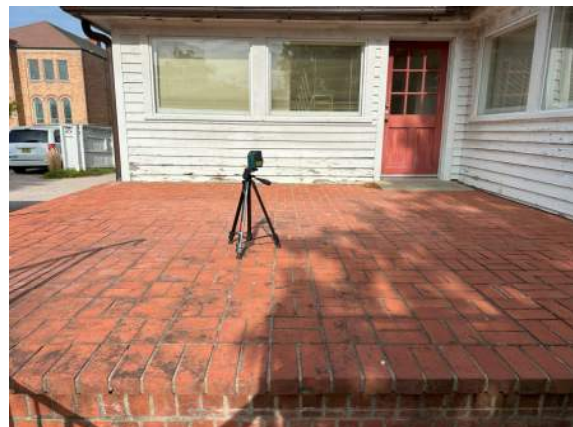
Picture 12 – Example of laser level set up for measurement of existing patio slab surface
