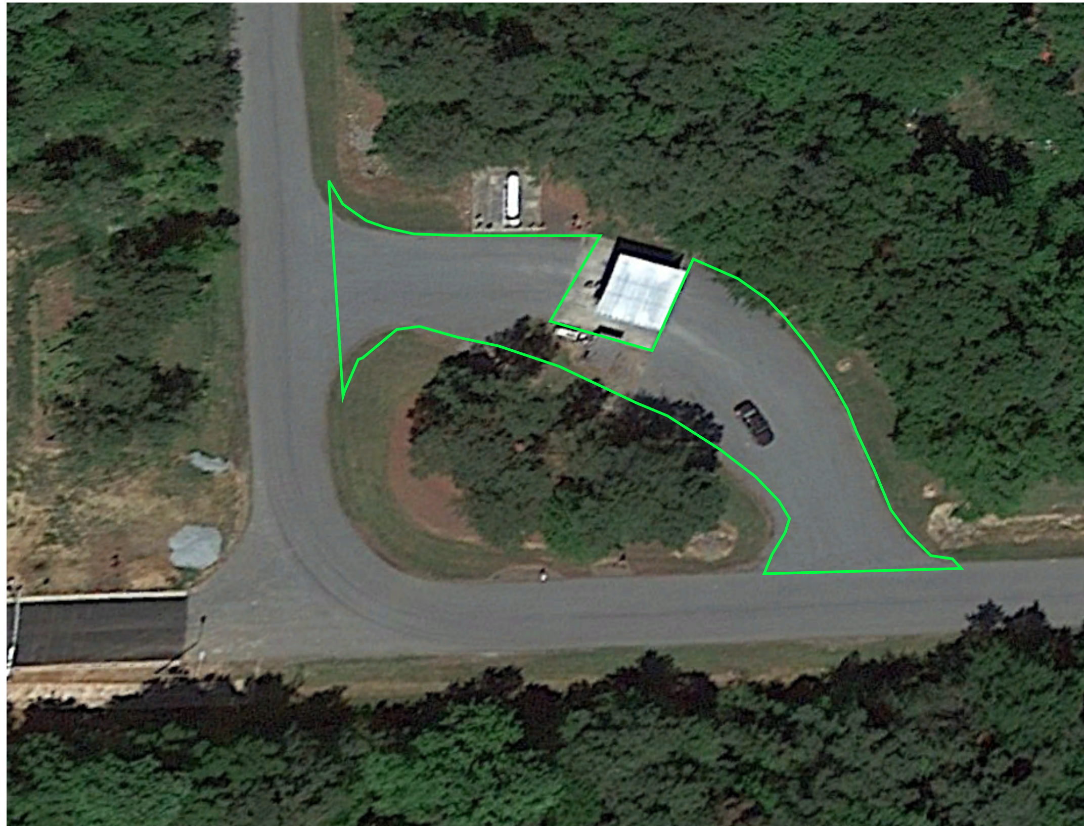
— Mill/Fill Asphalt Pavement 1.5" of Depth — Asphalt Surface Course, Type S9.5B at 1.5" of Depth
