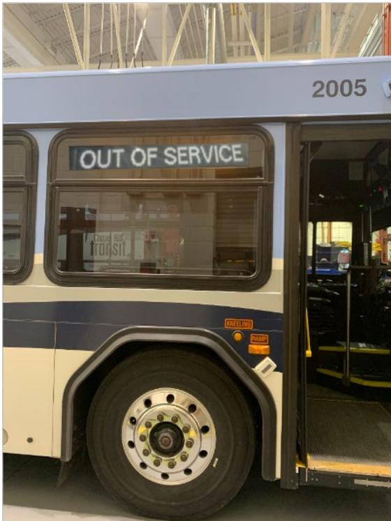
The Side Sign message shall be readable by a person with 20/20 vision, from a distance of not less than 110 feet. The Side Sign shall have a viewing cone of equal readability at 65 degrees on either side of a line perpendicular to the center of the mean plane of the display. The intensity of the illumination of the display pixels shall appear, to the naked eye, to be approximately uniform throughout the full viewing cone.
