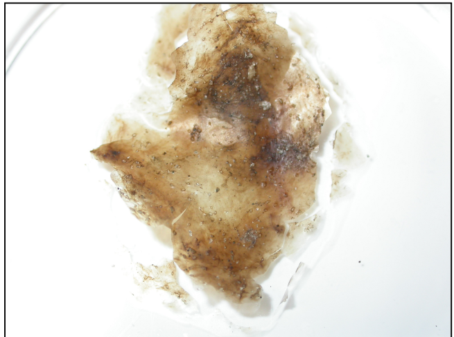
Figure 4: Macro of slime sample, after 24-hours of air-drying.
