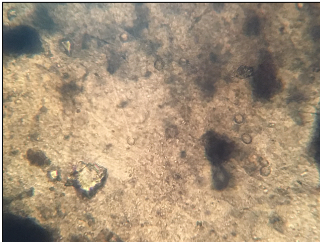
Figure 7: Heavy iron oxide entrained biomass with crystals and sporadic microbial cysts visible.
