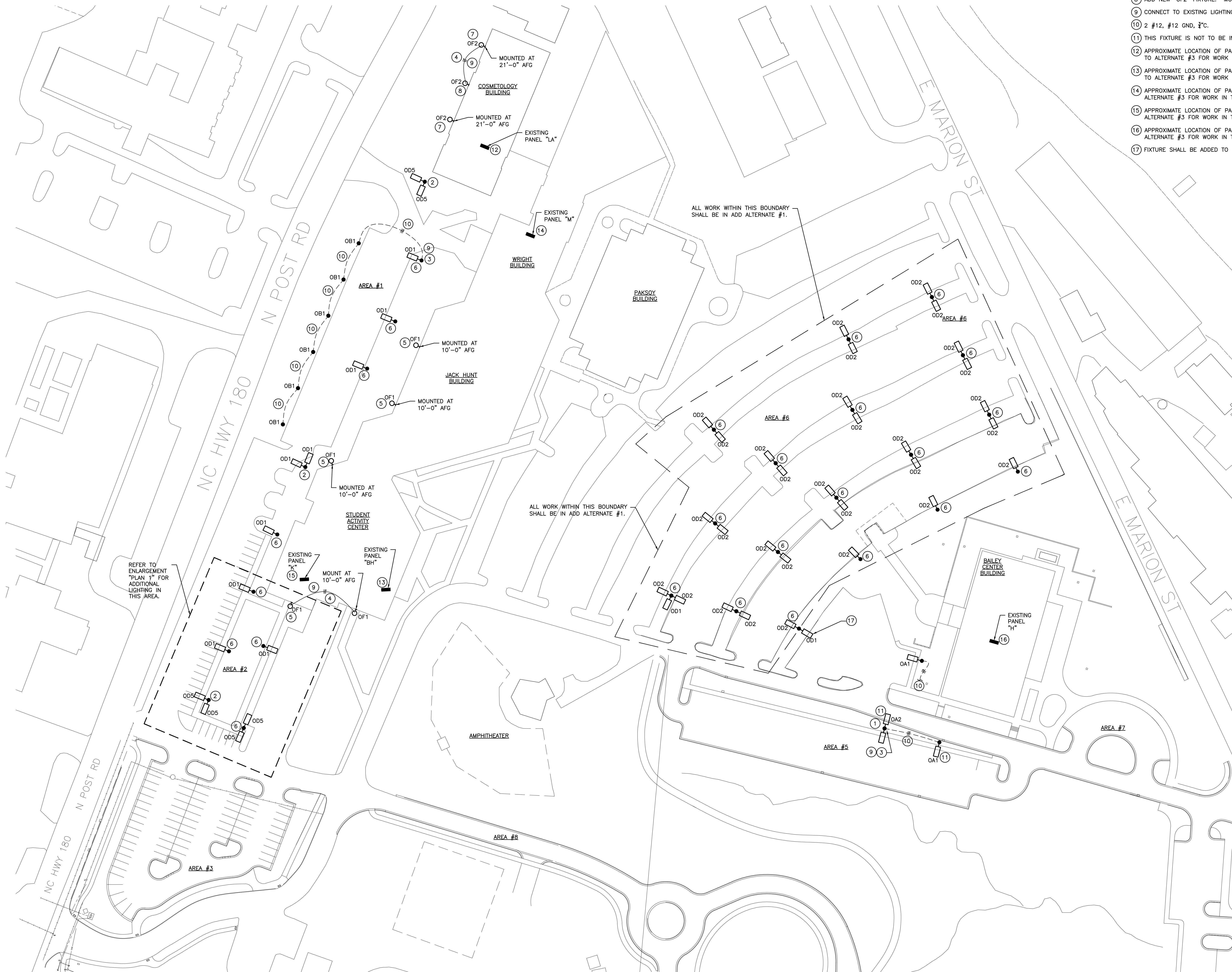
RENOVATED SITE PLAN - LIGHTING SCALE: 1" = 50'-0"
