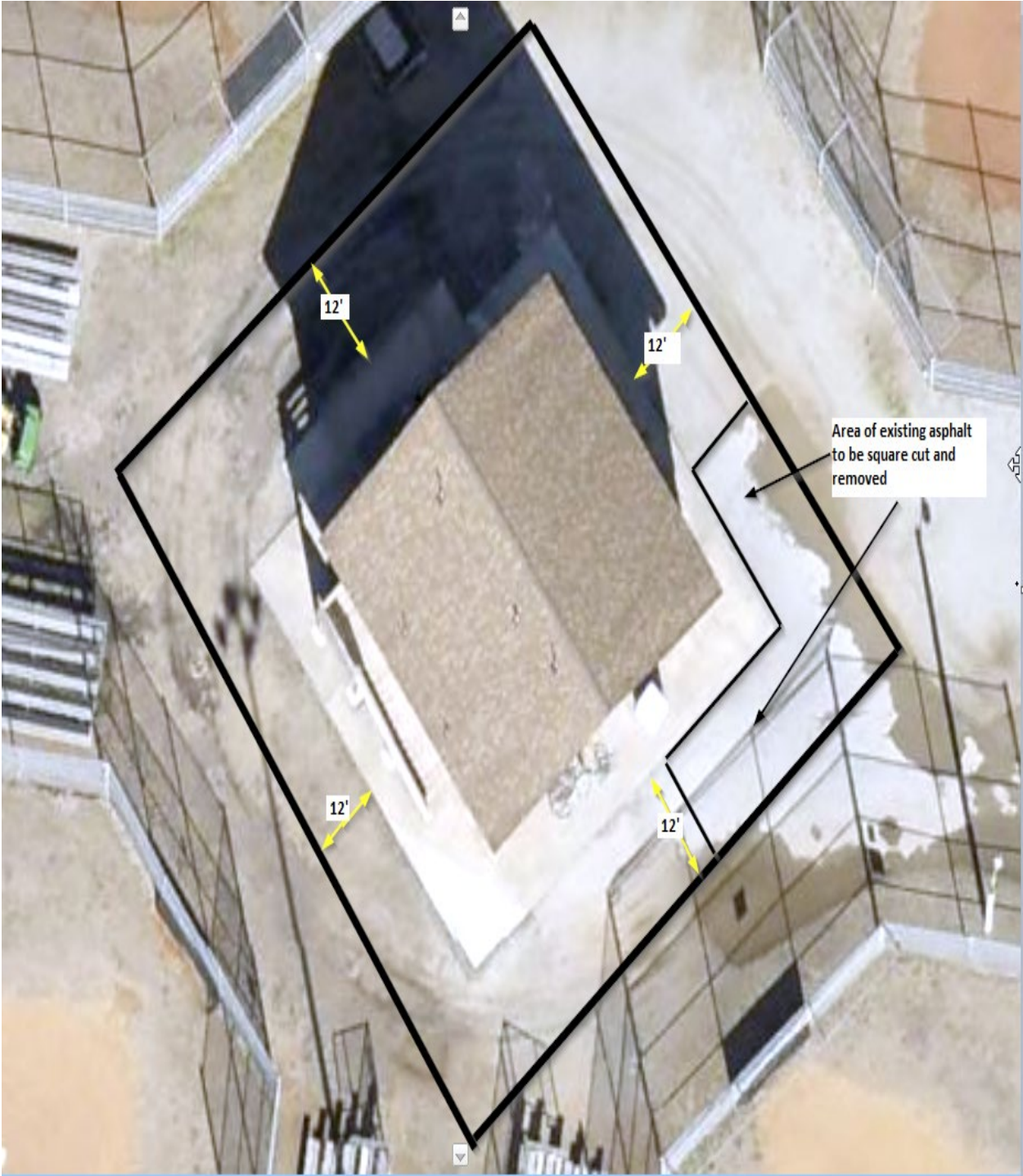
Figure 3: Line item #2 Asphalt to be installed around the Concession Stand
