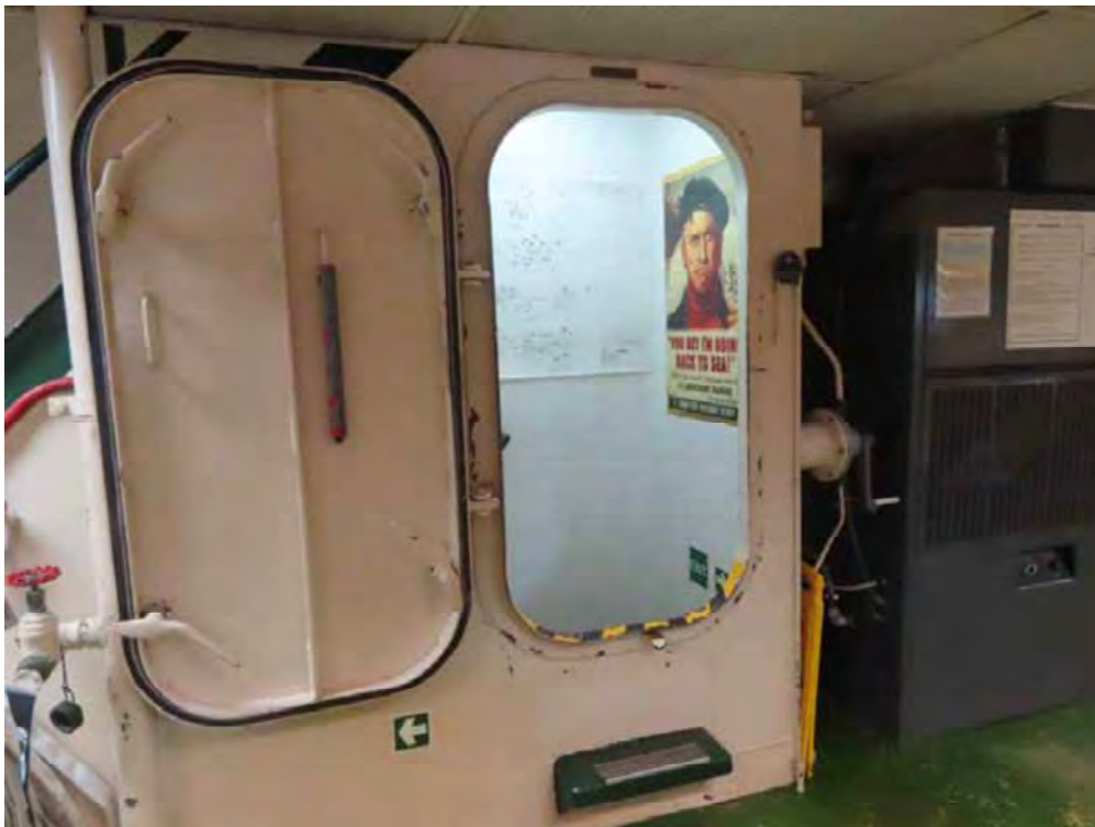
52. Watertight door in crew mess leading crew cabins and engine room
