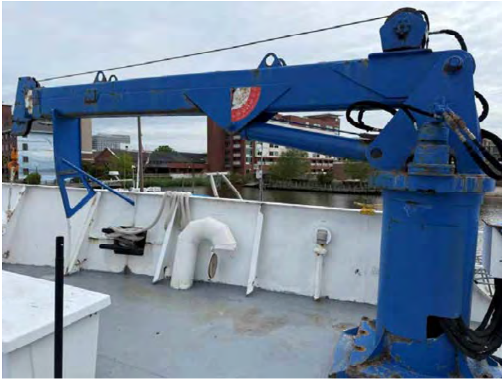
11. Cargo/Stores crane located on starboard side forecassle (reportedly out of certification)
