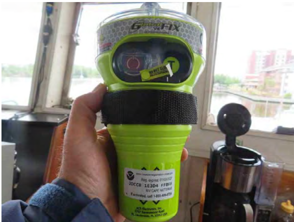
24. EPIRB located on bridge
