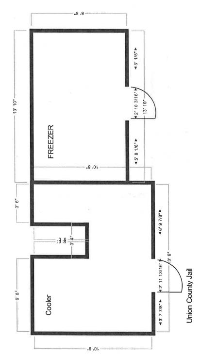
\*\* Preliminary Drawing Installer should verify dimensions prior to installation
