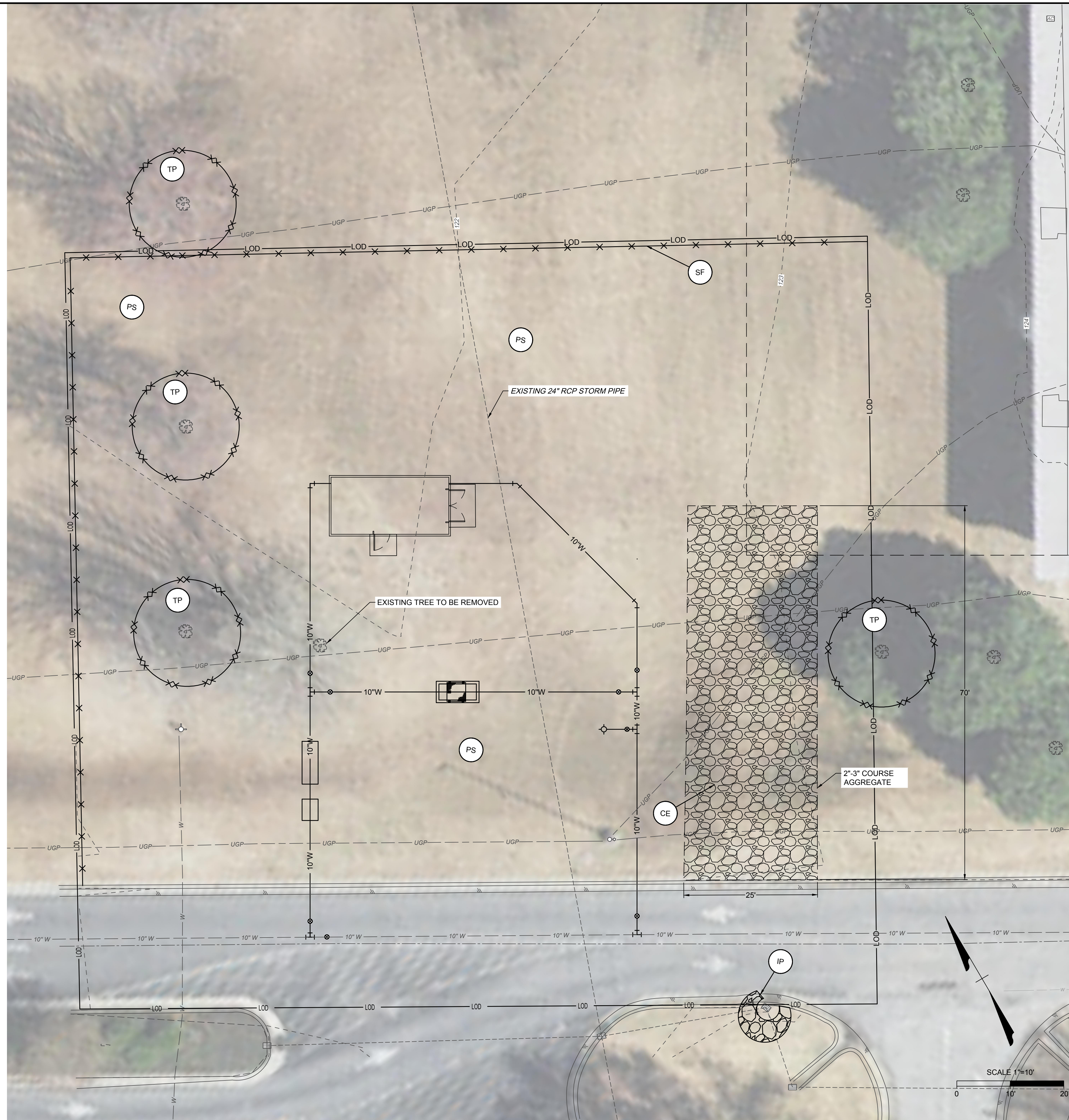
EROSION AND SEDIMENT CONTROL SITE PLAN SCALE: 1" = 10'
